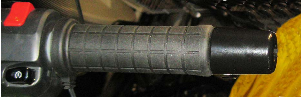
The installed throttle grip.
